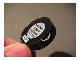
Start by breaking off the two plastic tabs on the sides of the casing with a pair of pliers.
