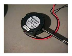
Use a thin edge (screw driver, xacto blade etc.) to gently pry the back plate off of the packaging. Careful not to bend the visible brass PZT disc
