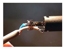
Tin both wires on the other end of the cable. Put two short pieces of heatshrink tubing on the PZT leads. Solder wires together. I prefer to do this by lining up two tinned leads side by side. Some people prefer to twist the wires together before tinning and soldering. Pull the heat shrink tubing back over the solder joints. Use a hair dryer to shrink the tubing over the joints. You're done. Go stick your contact mic on something, and call it art.
