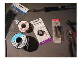
The functional element - a piezo electric transducer is commonly used as a speaker. Different models come in different plastic packaging, each more annoying to excise than the other. Do not buy the 12VDC versions - they cost more, and you'll end up throwing away the drive electronics anyway.
